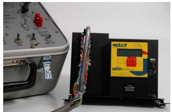
FIGURE 6, etc-12/etd Undergoing Test with Westinghouse Amptector Test Set
