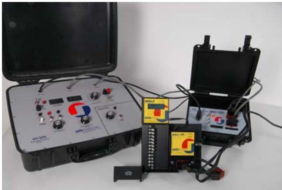
FIGURE 8, etc-12 Undergoing Test with the Satin American etc/pts with the pts adaptor
