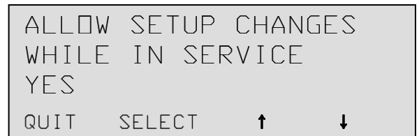
Figure 32, Enabling shunt trip from front panel
