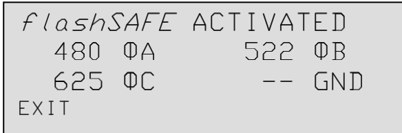
Figure 40, View of Display with flashSAFE Activated
