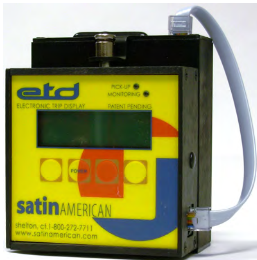
Figure 46, etd Nested on etc-12 for Breaker Mounting
